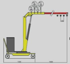
Mod.01B2 /01B2P comes with a revolving jib extendible in 4 positions
